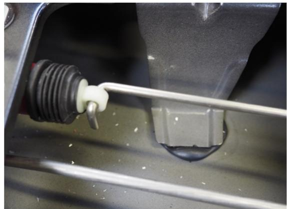
**5) Remove the Factory fitting Key Lock rod from the Vehicle**
