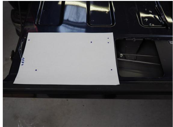
**3) Drill Holes for the motor, please use a 4mm Drill**
